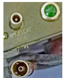
Close up view of the RF out socket on the Dutch collection and Blandford Polish test sets (left).
