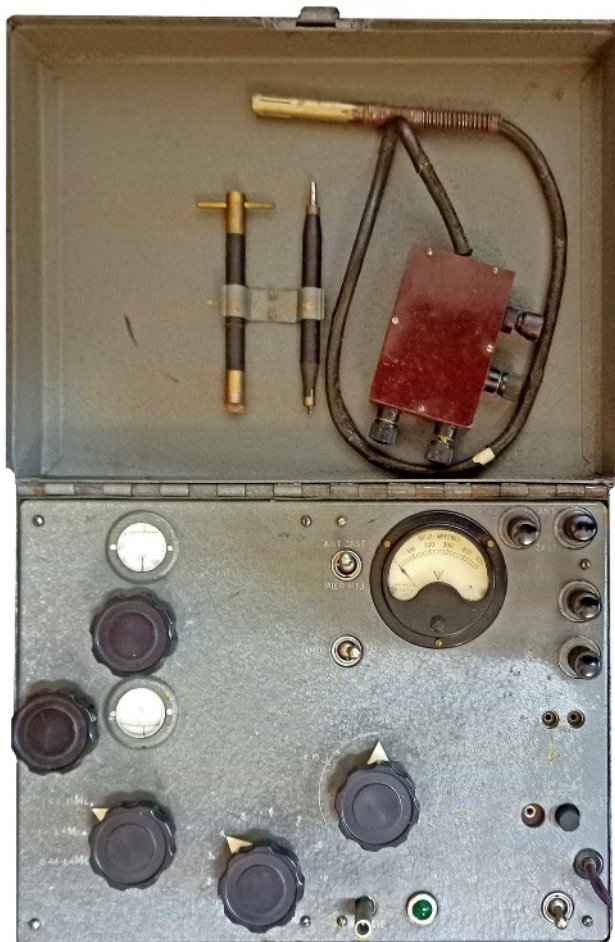
Photographs taken by Anthony Howard. His Polish test set is complete with both tuning tools and the signal generator artificial aerial. Note a different type of RF out socket and plug.
