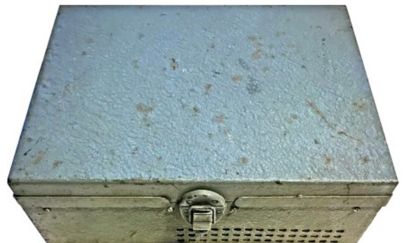
View of the Polish test set enclosure. Avoiding RF leakage of the signal generator, the (existing) punched ventilation holes were covered by metal plates at the inside.
