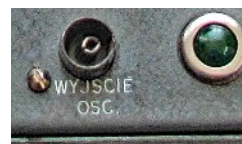
Close up view of the RF out socket on the Dutch collection and Blandford Polish test sets (left).
